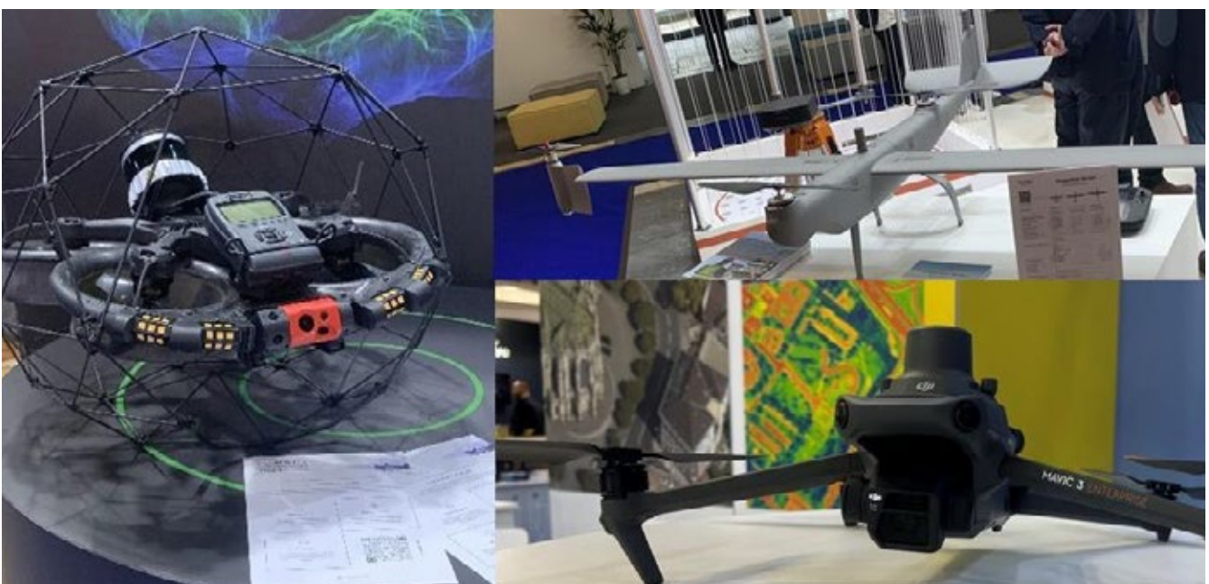
Collection of different systems (left: drone for indoor mapping; top right: drone with fixed wings, with a long flight time of up to 90 minutes and a high flight speed of up to 17 m/s; bottom right: small and compact drone).
