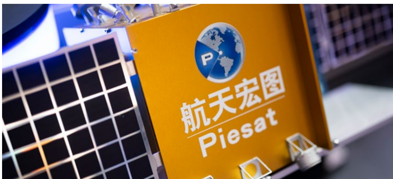
A model of the PIESAT 1A-01 InSAR satellite, which forms part of an InSAR constellation comprising active and passive X-band SAR satellites. The constellation will provide data with a resolution of up to 0.5 m for the investigation and early detection of significant geological hazards such as subsidence, collapses and landslides.
