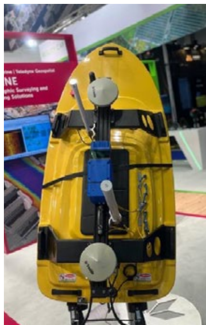
On the left is a drone solution for bathymetric surveying and on the right a service vehicle for hydrology applications.
